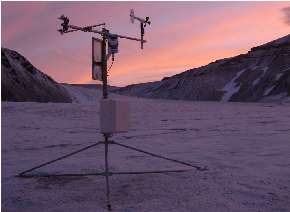
Fig. 4.3 Automatic weather station on Svenbreen in autumn 2011
