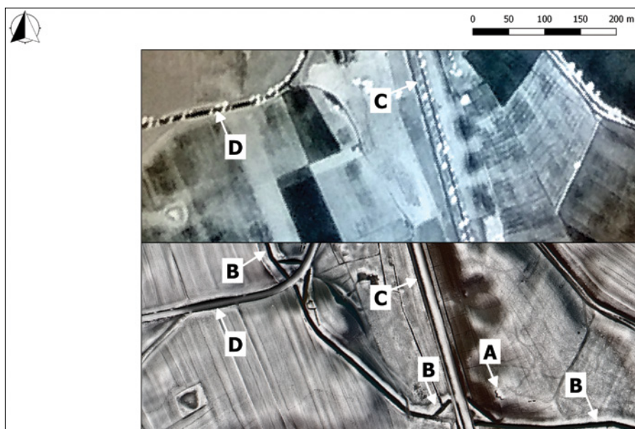
Figure 68. While infantry trenches (A) and the anti-tank ditch (B) are clearly visible next to the roads connecting Polanów with Żydowo (C) and with Łokwica (D) in the ALS-derived DTM visualization (bottom), there is no trace of the fortification on the reconnaissance photograph taken by United States Air Force in 1944 (top). National Archives and Records Administration: photograph no. 4349, roll D13971-D13973. ALS-derived DTM visualization: local dominance superimposed on sky-view factor and hill-shading from multiple directions (Red – channel 14; Blue – channel 1; Green – channel 3).
