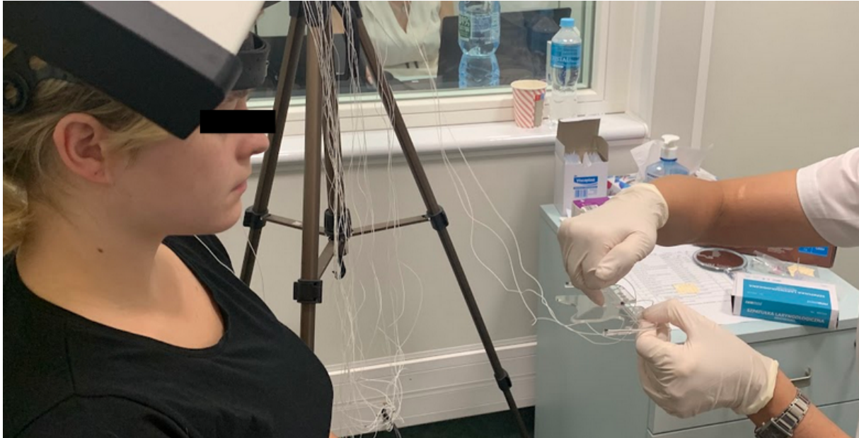
Figure 3.6. Preparation for placing biteplane in the participant's mouth. All the procedures involving physical contact with participants and equipment were performed in sterile latex surgical gloves.
