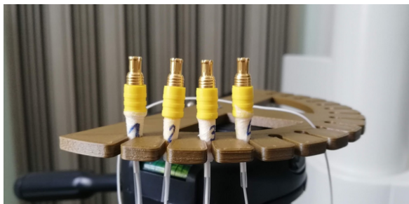
Figure 3.8. Electromagnetic sensors mounted in a wooden calibration holder. Four sensors are shown with their cable connections and marking, enabling precise use in the AG501 articulograph system.
