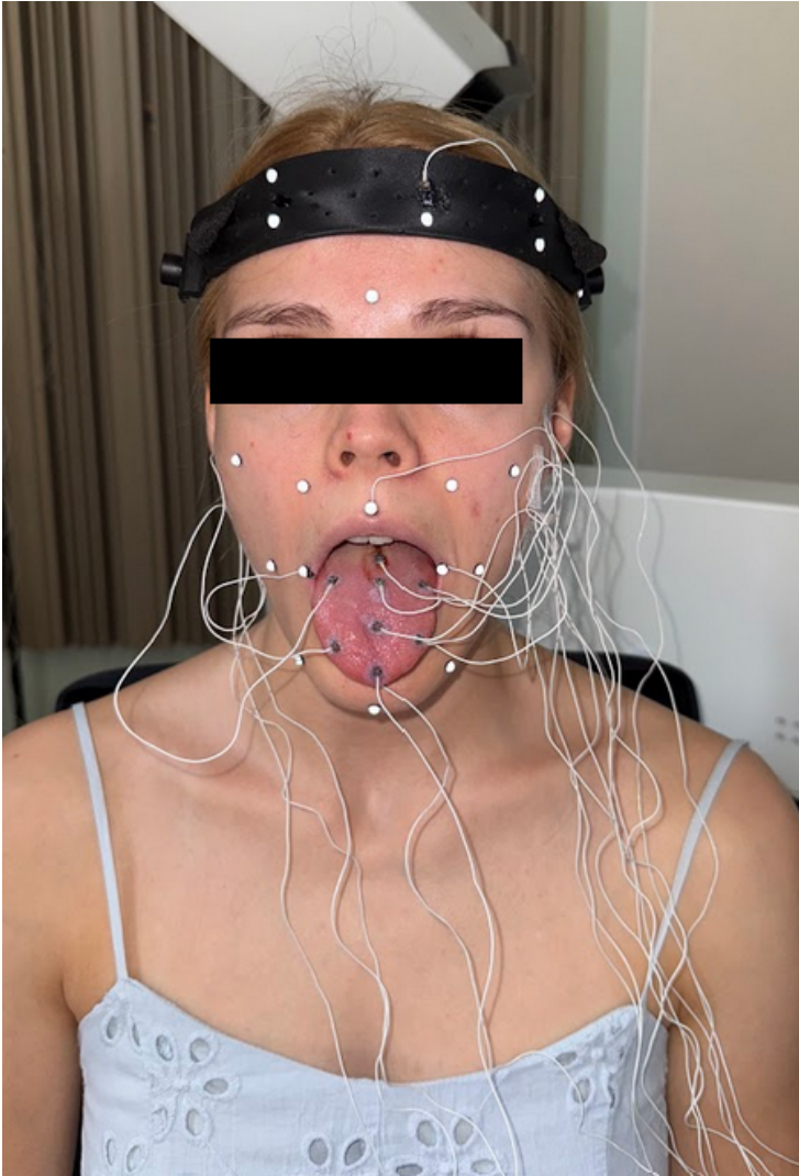
Figure 3.2. Example of EMA sensor placement – the upper lip sensor is clearly visible.
