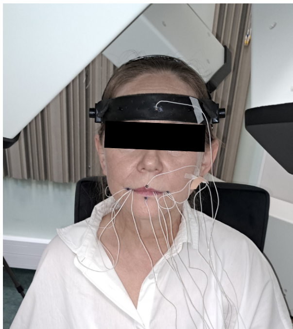
Figure 3.5. A speaker prepared for an Electromagnetic Articulography (EMA) recording session using the Carstens AG501 system. Receiver sensors are already attached. The subject is wearing the reference coil headband, with transmitter coils visible in the background, which generate the alternating magnetic field used for tracking sensor coordinates.
