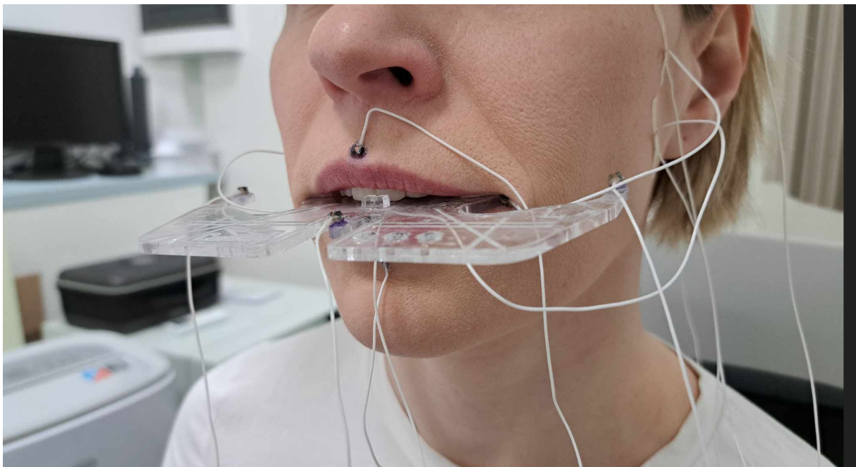
Figure 3.7. The biteplane, held between the participant's teeth, serves multiple functions, including providing a fixed reference point for the measurement system.
