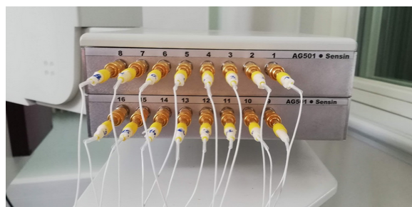
Figure 3.9. Electromagnetic sensors connected to the AG501 Sensin receiver unit. Each sensor is plugged into its numbered port according to the calibration protocol, ready for articulographic data acquisition.
