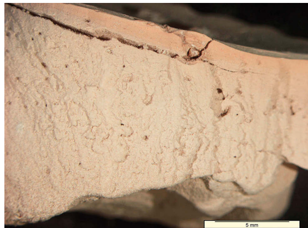
Fig. 204. Specimen P029 after firing at 600°C
