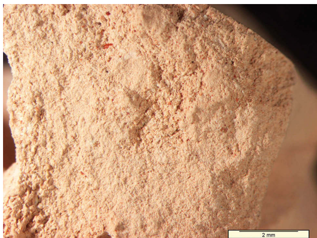
Fig. 211. Specimen P.253 – Taqiye marl after firing at 600°C
