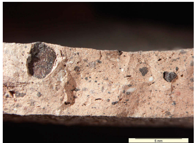
Fig. 145. SG.IV.E. Specimen TK-200, photomicrograph of a fresh break
