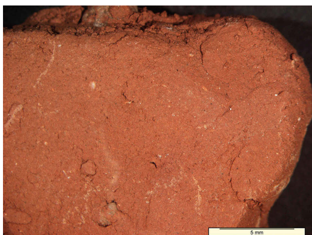
Fig. 199. Specimen P27 after firing at 650°C
