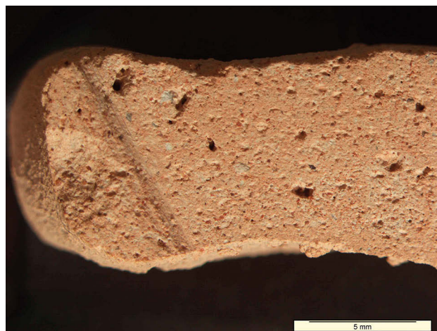
Fig. 205. Specimen P33H: a vessel made by mixing the P.033 marl with hamra soil and terra rossa
