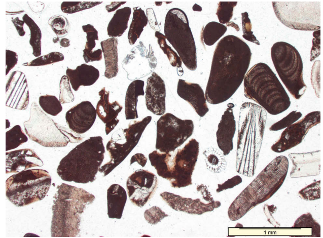
Fig. 230. Specimen P-2, Nahariya, central beach sands, photomicrograph of a thin section (PPL). The only component is organogenic detritus, including such microorganisms as Ammonia sp., Astergerina sp., Miliolidae , as well as numerous fragments of Corallinacea and snails – an association diagnostic for the Late Eocene
