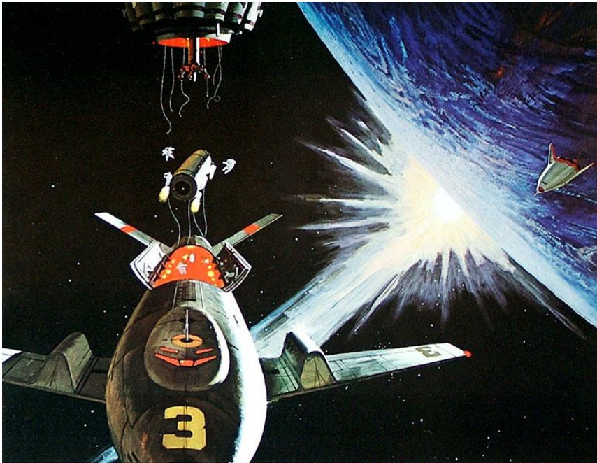
Caption: A shuttle in Earth orbit deploying its payload. The cargo has its own little thrusters for controlling attitude; these are operated by the astronaut at its right working at an external control panel. The tethers at the top of the painting extend from a space station that uses the shuttle system to replenish supplies.
