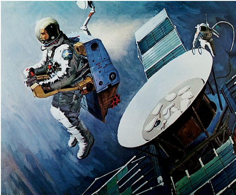
Caption: Skylab crewman testing astronaut maneuvering unit. (The unit was tested inside Skylab, although it is intended for exterior use; courtesy of artist's license, it is shown that way here.) At right is the Apollo telescope mount surrounded by the four solar wings that were the principal source of solar power for Skylab before the crippled panel was deployed.
